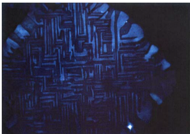
Figure 1. Single crystal of BP II after cooling into BP I (from [13]).
